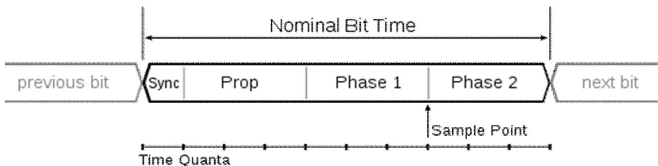
An example CAN bit timing with 10 time quanta per bit.
