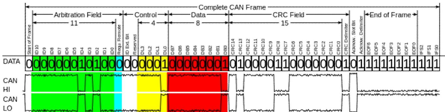
CAN-Frame in base format with electrical levels without stuffbits
