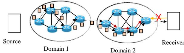
Fig. 11. If receiver don't send feedback then nearly boundary router send INITIATION message again
