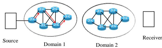
Fig. 13: Ingress node send test message to egress node to check ingress-to-egress node connectivity in a domain
