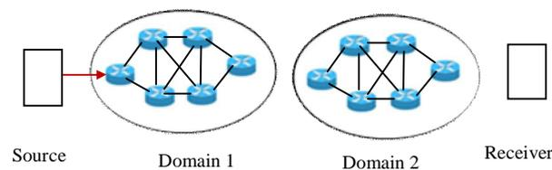
Fig. 3 sender sends data packets to boundary router via ISP
