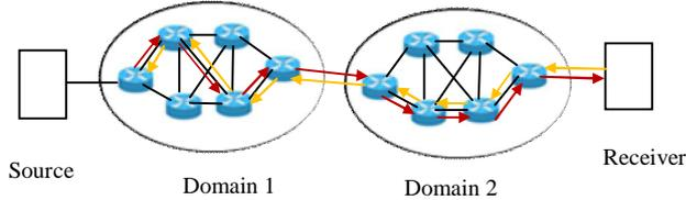
Fig. 7 Receiver gives a feedback to the boundary router
