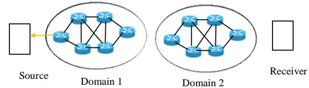
Fig. 14: If feedback doesn't come, boundary router drops packet and sends a message to source to stop transmission
