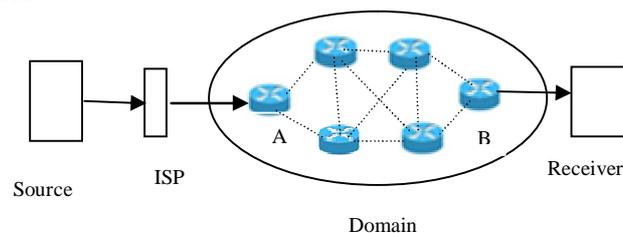
Fig. 1 A, B are boundary router in a domain. In between A & B 4 core router are present. Path are created between A to B by first fit method.
