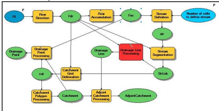
Fig. 3 Model Builder for Delineate Catchment
