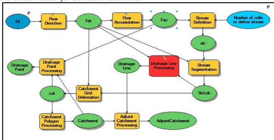
Fig. 3 Model Builder for Delineate Catchment
