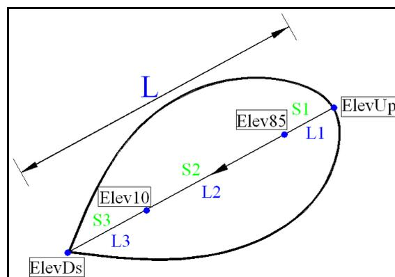
Figure (7) Longest Flow Path Divisions According to Length
