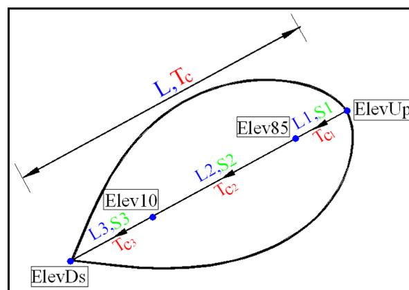
Fig. 10 Longest Flow Path Divisions According to Time of Concentration
