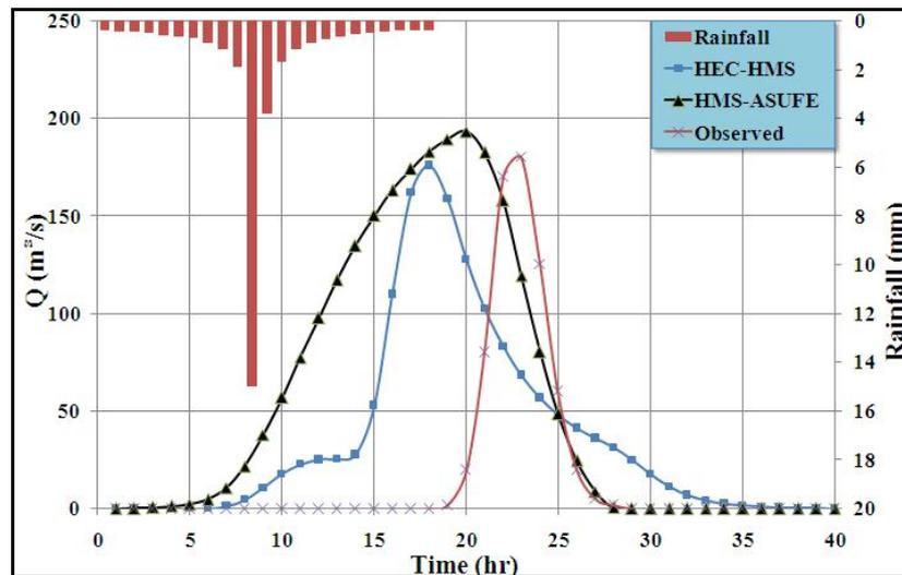
Fig. 15 Runoff Hydrographs and Rainfall at Outlet Using HEC-HMS, HMS-ASUFE by SCS Type 2, and Observed Hydrograph
