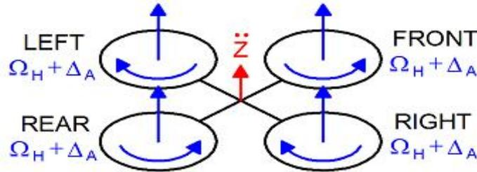
Fig. 3 Throttle command on a Quadcopter
