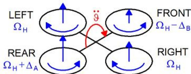
Fig. 5 Pitch command on a Quadcopter
