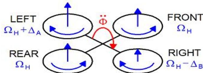
Fig. 4 Roll Command on a Quadcopter
