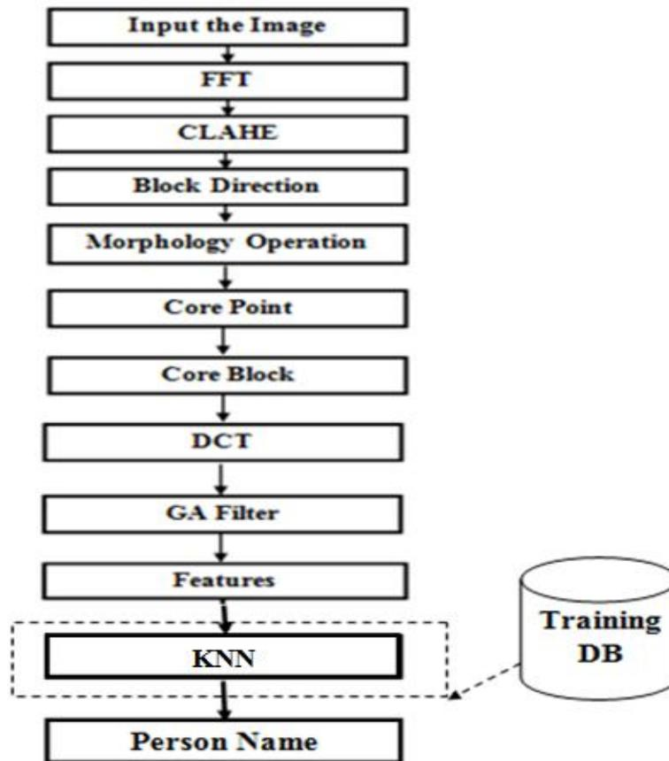
Fig. 5 Block diagram of the identification phase in proposed method.
