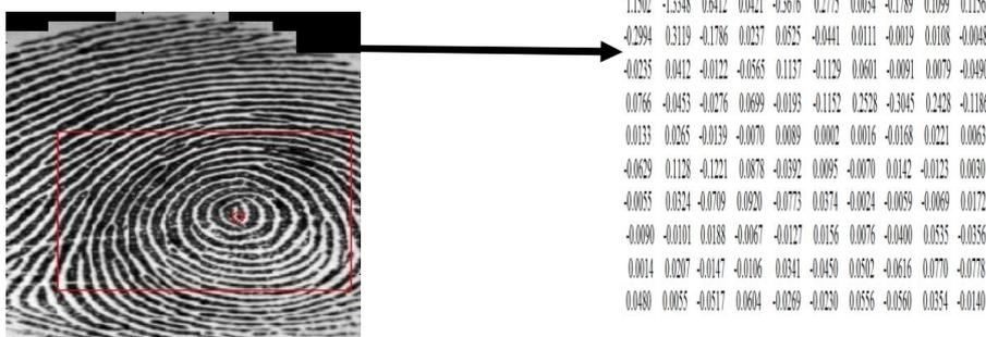
Fig. 4 Show feature vector that out from DCT.
