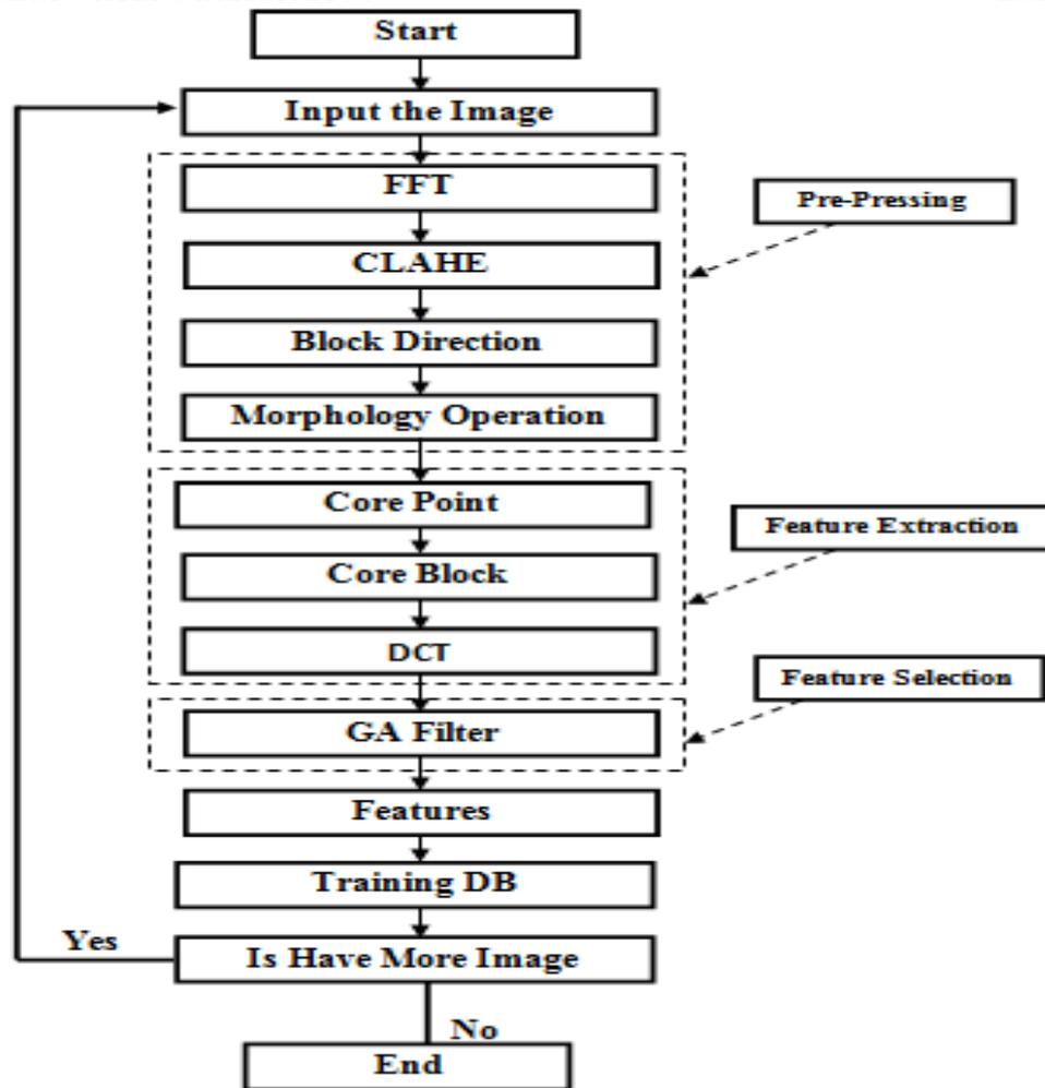
Fig. 1 Block diagram of the feature extraction phase in proposed algorithm.
