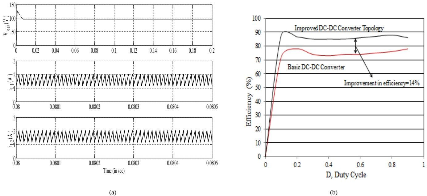
Fig. 6. (a) Output voltage, inductor current through L1 and inductor current through L2 at 100kHz, 12-100V operation, (b) Efficiency curves of basic and improved topology for different values of duty cycle
