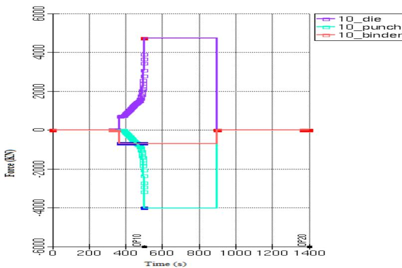
Fig.4 Diagram of forces in the forming process
