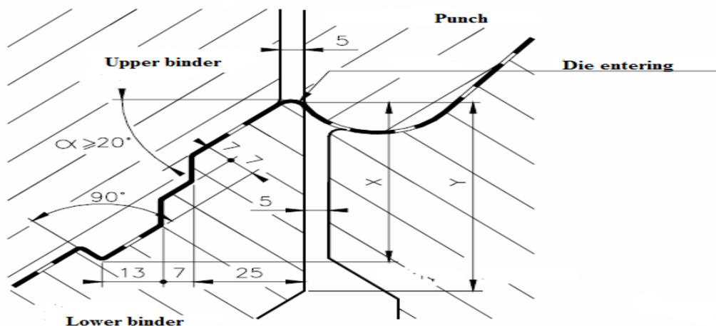
Fig.3 The case when binder surface has a slope  $> 20^\circ$
