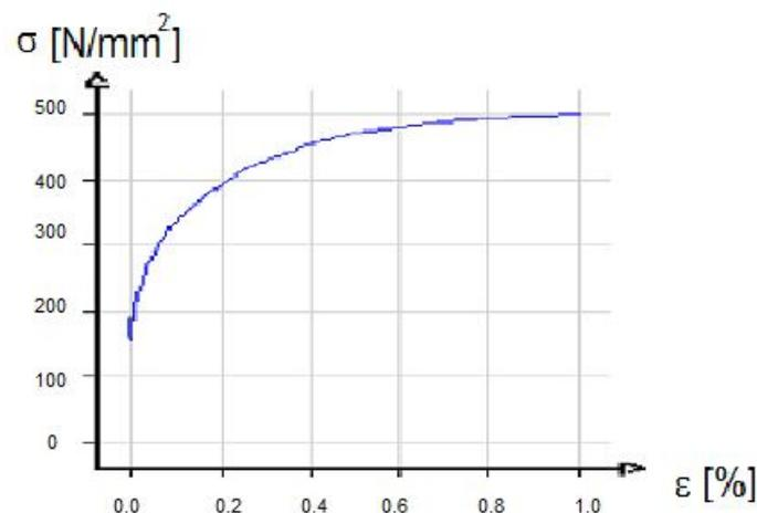
Fig.1 The characteristic curve for the material DC 04
