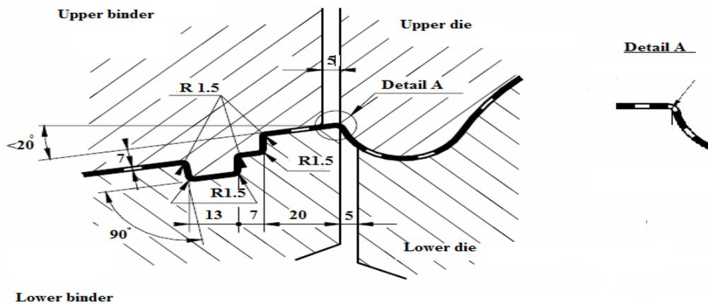
Fig.2 The case when binder surface has a slope  $0^\circ - 20^\circ$
