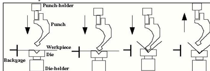
Figure 2. Bending process phases as in [8]
