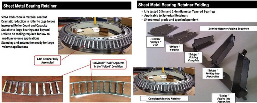
Figure 4 Industrial Origami Bearing Retainers as in [8]
