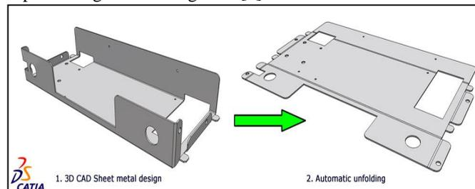
Stage 1: Designing and Unfolding
