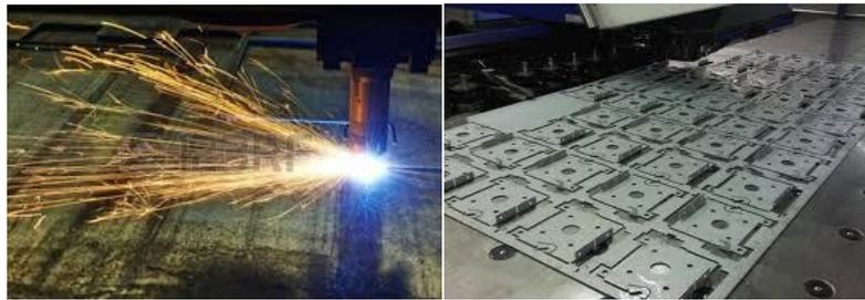
Stage 2: Flat Processing (Punching, Laser)
