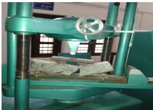
Fig. 4 Crack pattern in the beam without and with steel fiber
