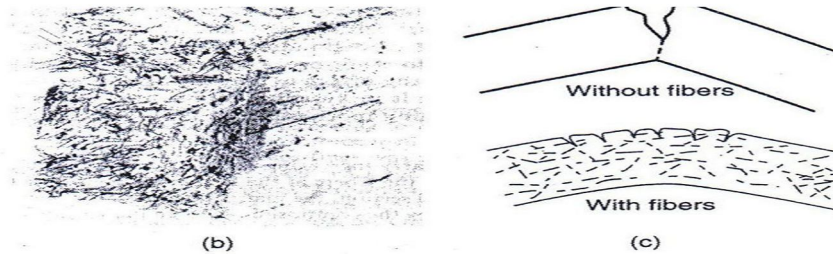
Fig. 1 Failure mechanism and the effect of fibers
