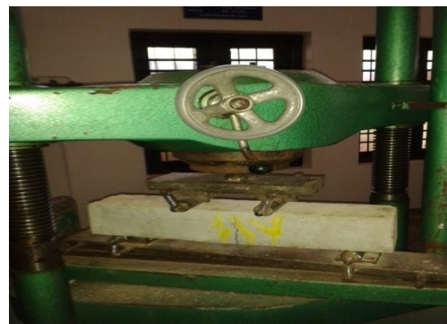
Fig. 4 Crack pattern in the beam without and with steel fiber
