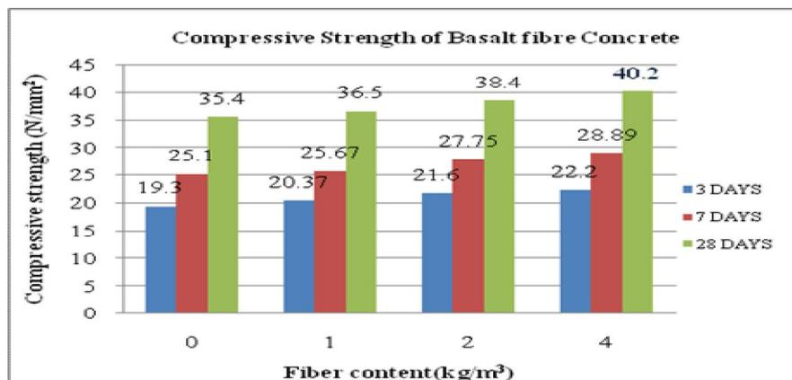
Fig: 2 Compressive strength of basalt fiber specimens
