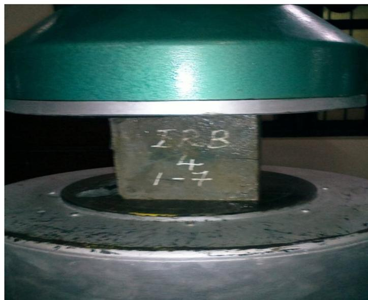
Fig: 3 Test for Compressive Strength
