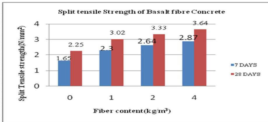
Fig: 4 Split Tensile strength of basalt fiber specimens
