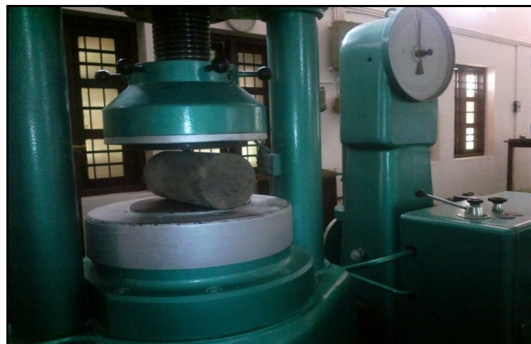
Fig: 5 Test for Splitting Tensile Strength
