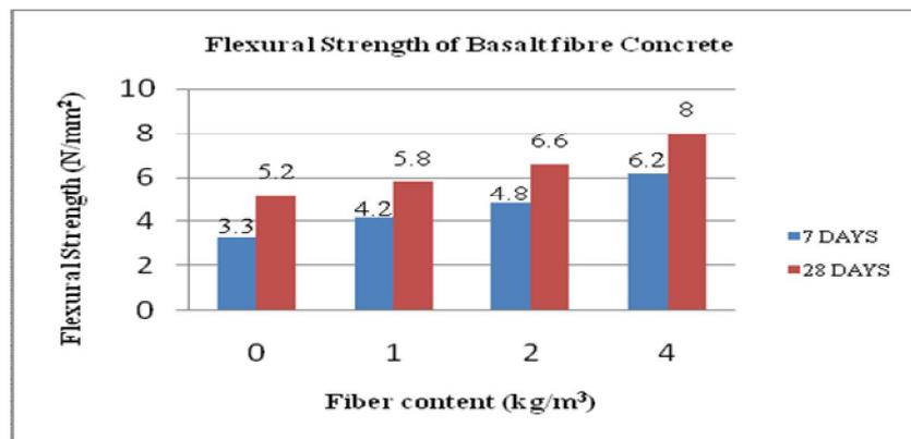
Fig: 6 Flexural strength of basalt fiber specimens
