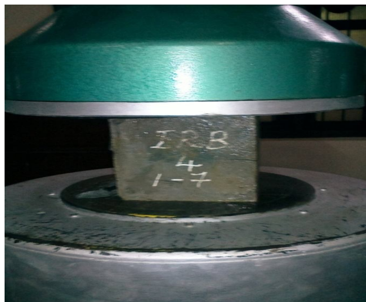
Fig: 3 Test for Compressive Strength
