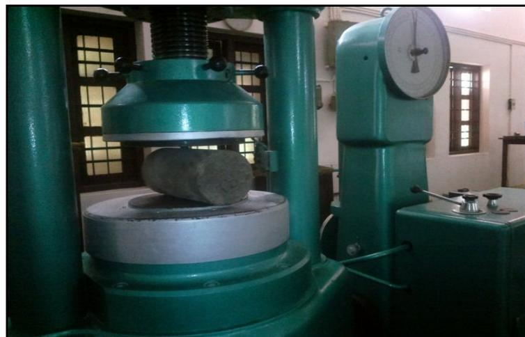
Fig: 5 Test for Splitting Tensile Strength
