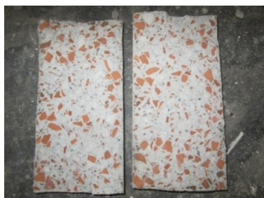
Fig. 3Cylinder with 100 % tile aggregate
