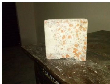
Fig. 1 Cube with 100 % tile aggregate
