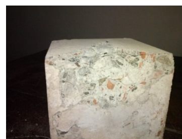
Fig. 2 Cube with 50 % tile aggregate
