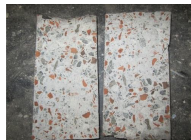
Fig. 4 Cylinder with 50 % tile aggregate
