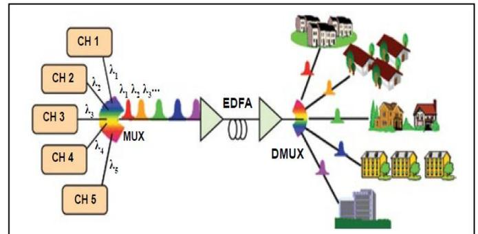
Fig. 1. Block diagram of DWDM system.
