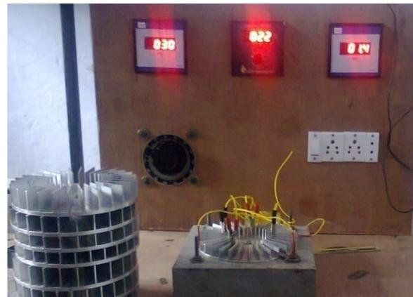
Fig. 1. Radial heat sink with a circular base and rectangular fins & experimental setup.
