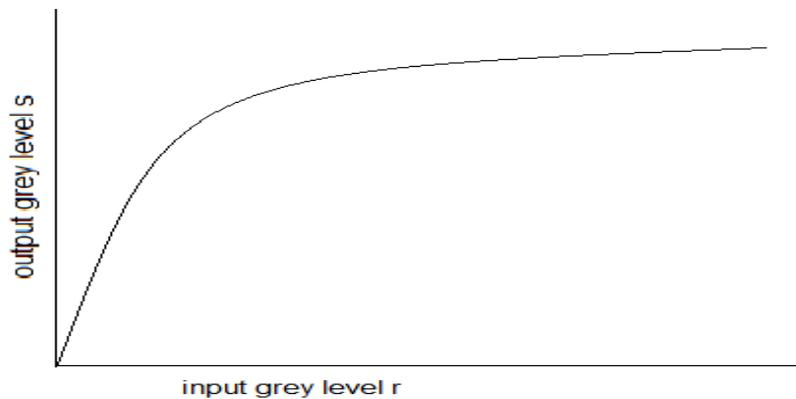
Fig.3 Log Transformation Curve
