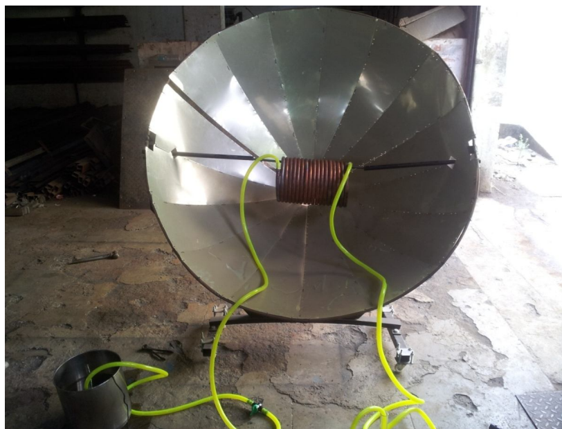
Fig 1 Parabolic dish concentrator experimental setup.
