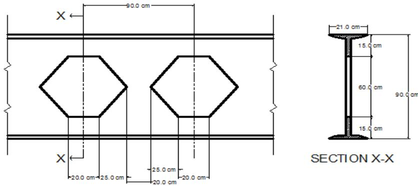
Fig. 2 Cross Section of Castellated Beam [4]
