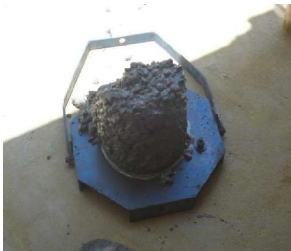
FIG. 4: SLUMP CONE TEST
