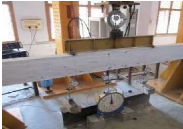
Fig.3 Testing of RC Beam in the laboratory
