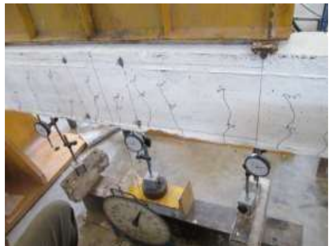
Fig.5 Crack Pattern of RC Beam
