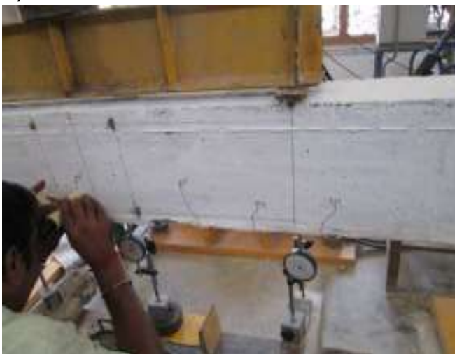
Fig.4 First Crack of RC Beam
