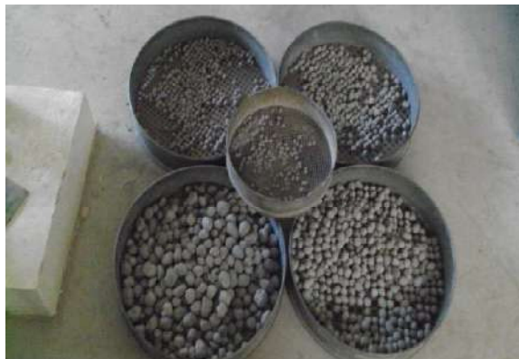
Figure 3.2. Segregation of fly ash aggregates.
