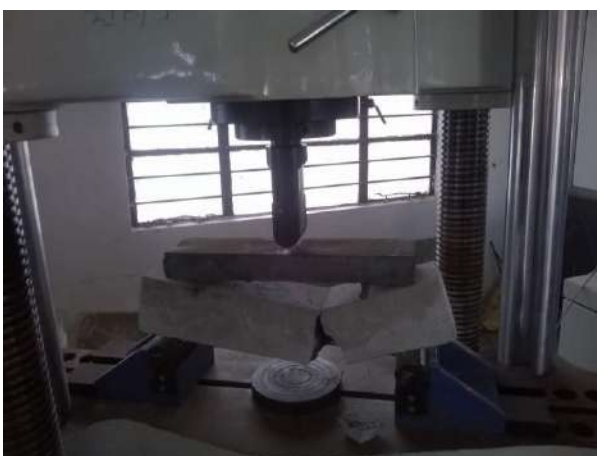
Fig 5.7 Testing of Prism for Flexural Strength in UTM
