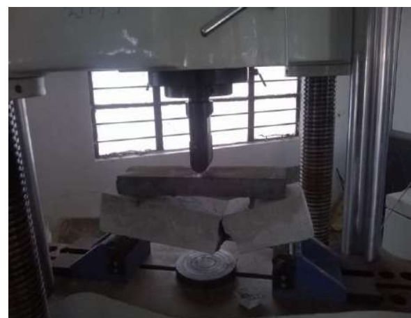
Fig 5.7 Testing of Prism for Flexural Strength in UTM
