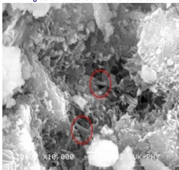
Fig 6.7 SEM Picture of Fly Ash Concrete Showing Bacterial Induced Calcite Deposition in Micro Cracks
