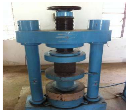
Fig Testing of Cubes in CTM
