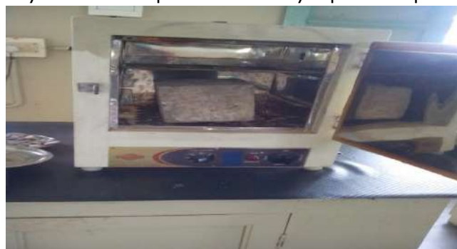
Fig. 17 Water Absorption Test
