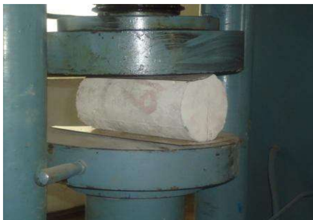
Figure 4.3 Failure Of Cylinder Specimen
