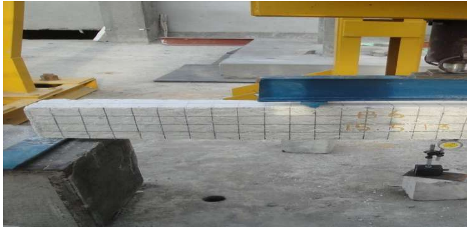
Fig 3.7 Test setup for Beam specimen
