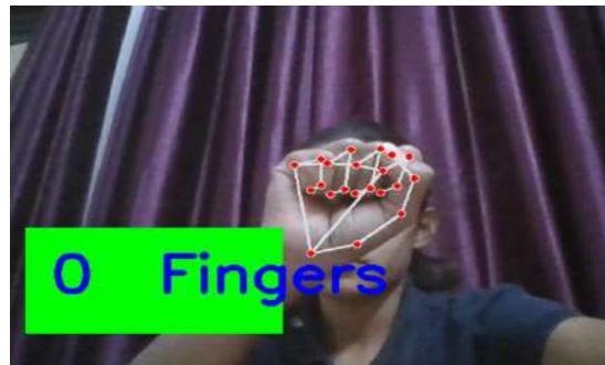
Fig 2: -When no fingers were raised to turn the light OFF.
