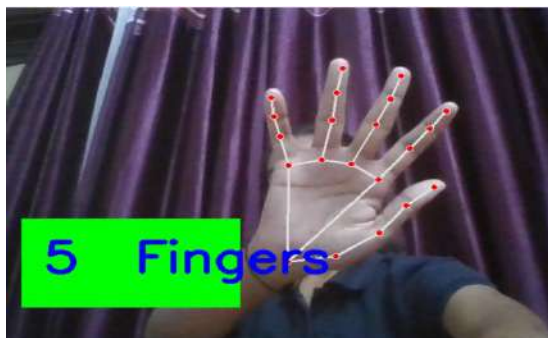
Fig 3: -When all fingers were raised to turn the light ON with full brightness.
