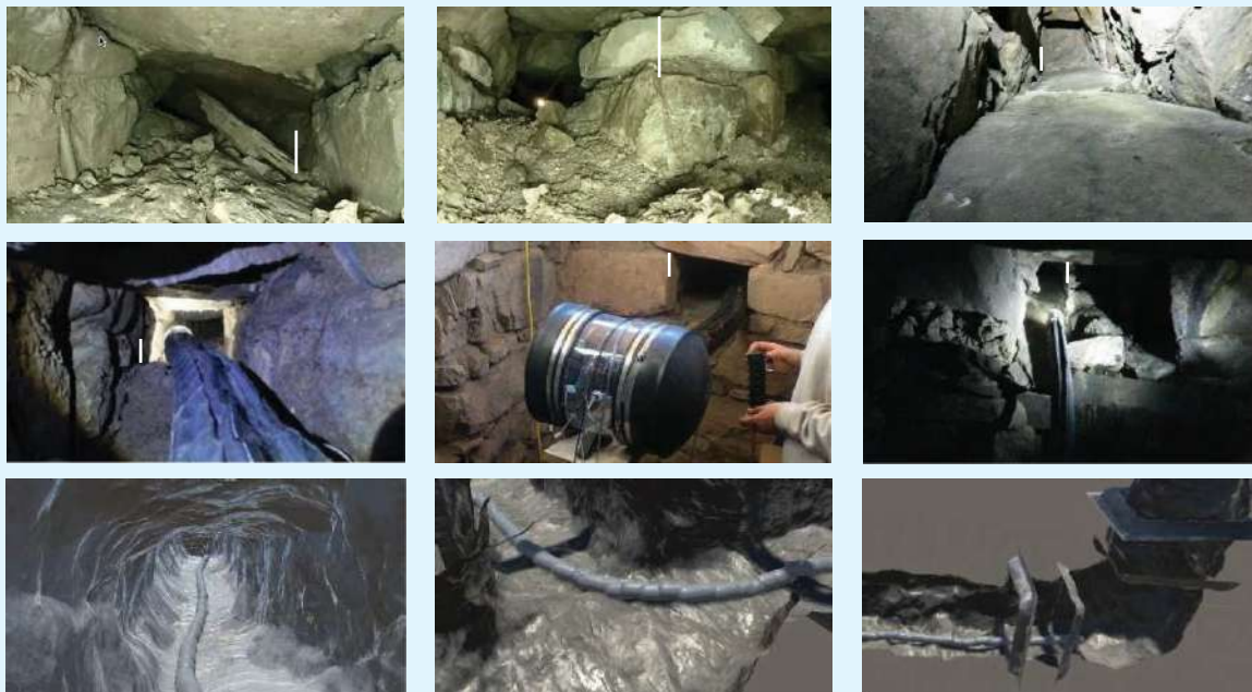
Figure 9. The map, photos, and simulation images of the vine robot's successful exploration of underground tunnels in an archeological site in Chavin, Peru. (a) A map of the archeological site. Areas the vine robot explored are marked in purple. (b) Location 1: a tunnel nearly blocked by rocks. (c) Location 2: a tunnel with a 90° right-hand turn. (d) Location 3: a tunnel that slopes upwards and then turns vertically. Top row: photos from inside the tunnels; middle row: photos of the vine robot in the tunnels; bottom row: screenshots of the simulation of the vine robot in each tunnel.
