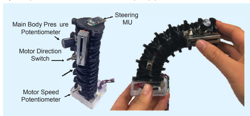
Figure 5. The flexible joystick used for teleoperation. The joystick contains switches and sensors to control the motion of the soft robot body.
