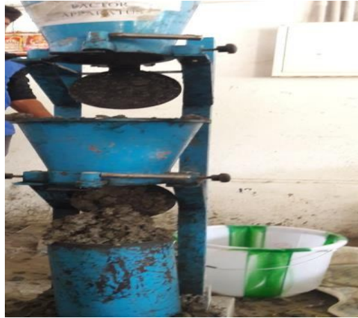
Fig: Compaction factor test
