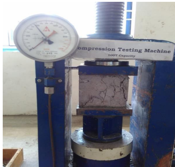
Fig: Compression testing
