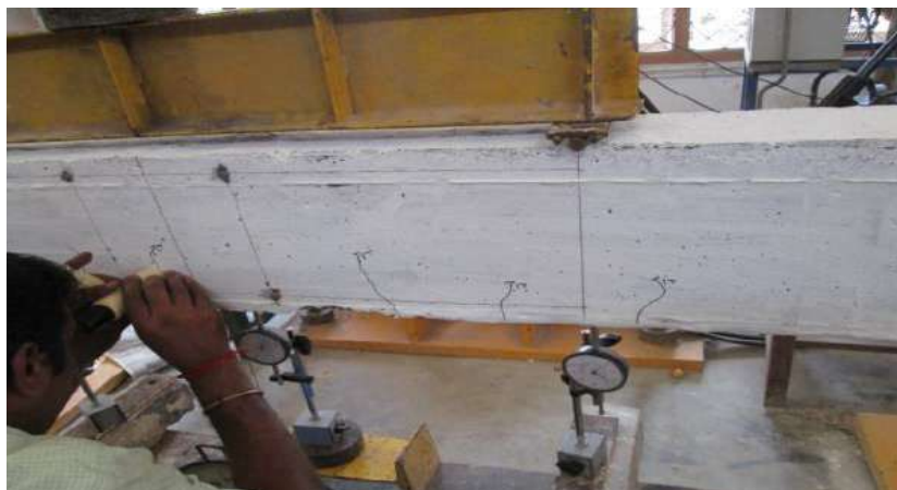
Fig.3 Testing of RC Beam in the laboratory
