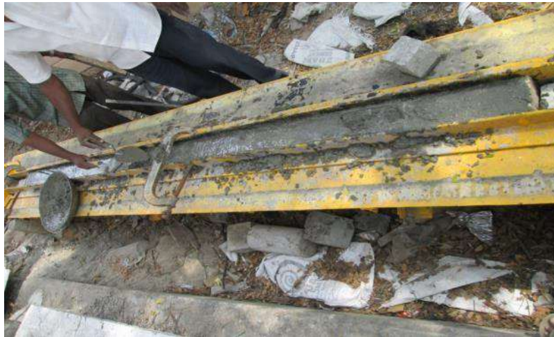
Fig 2 Casting of Reinforced concrete beam in the laboratory
