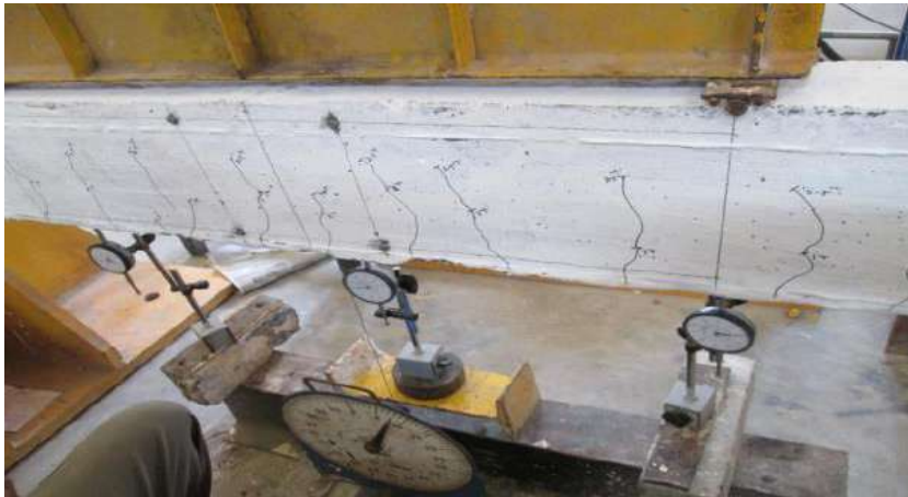
Fig.4 First Crack of RC Beam
