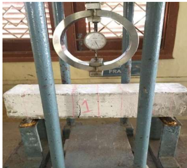
Fig.7 Failure of prism specimen
