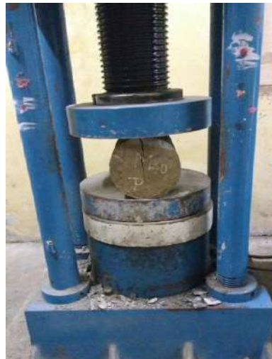
Fig.6 Failure of cylindrical specimen
