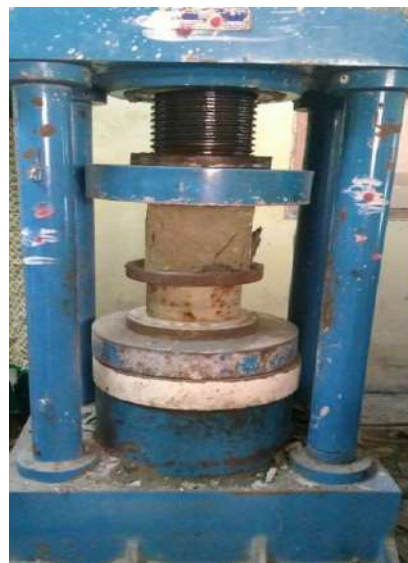
Fig.5 Failure of cube specimen
