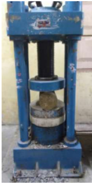
Fig.4 Testing of concrete prisms
