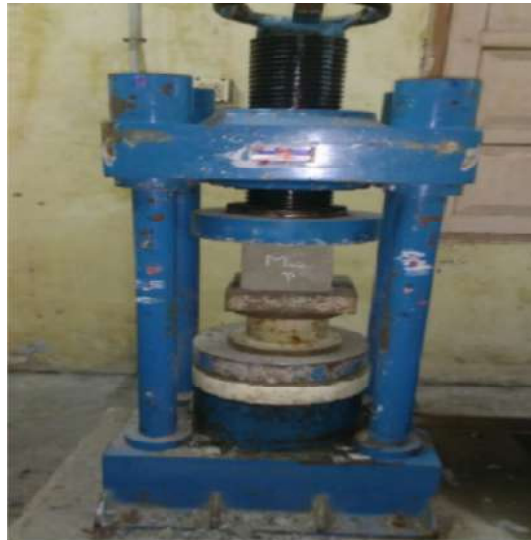
Fig.3 Compression test on concrete cubes
