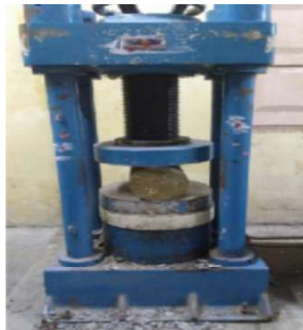
Fig.4 Testing of concrete cylinders
