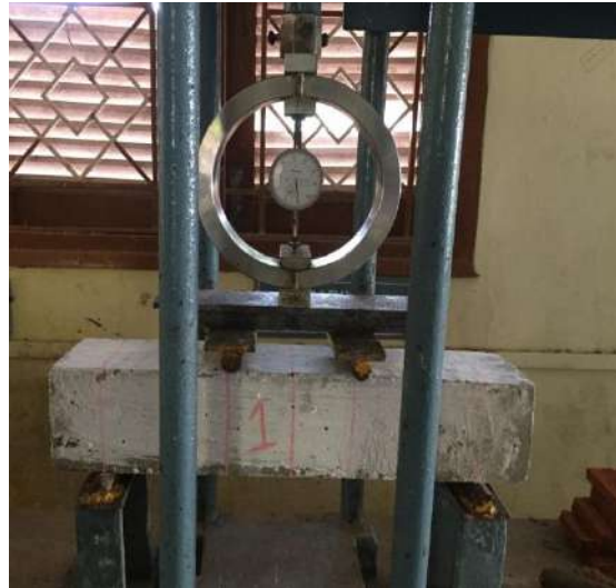
Fig.4 Testing of concrete prisms
