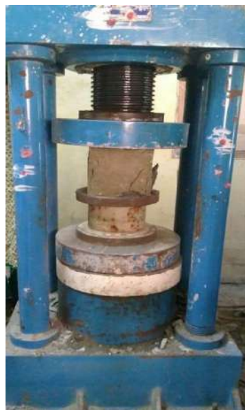
Fig.5 Failure of cube specimen
