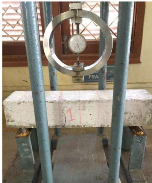
Fig.7 Failure of prism specimen
