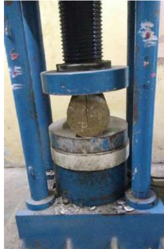
Fig.6 Failure of cylindrical specimen
