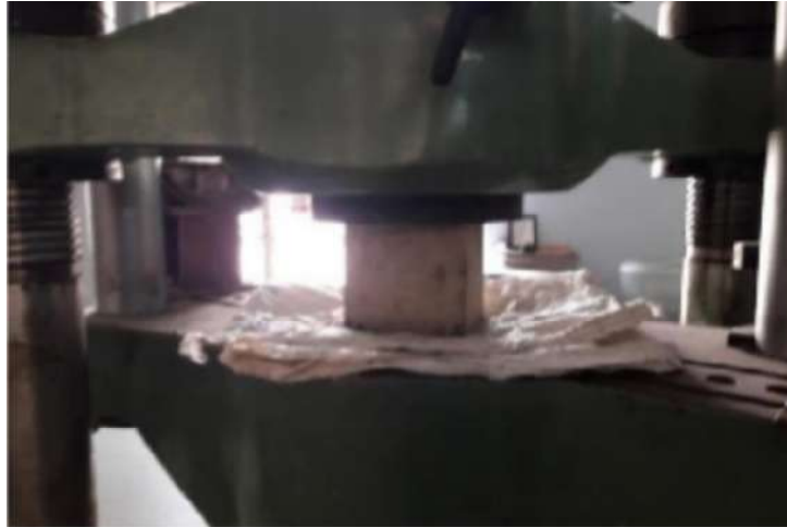
Fig.4.1 Testing of cubes in UTM Table 4.1 Values of Compressive Strength test
