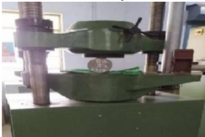
Fig.4.2 Splittensile test on concrete cylinder
