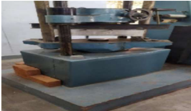
Fig. 4.3 Flexural Strength test on prism Table 4.3 Values of Flexural Strength test
