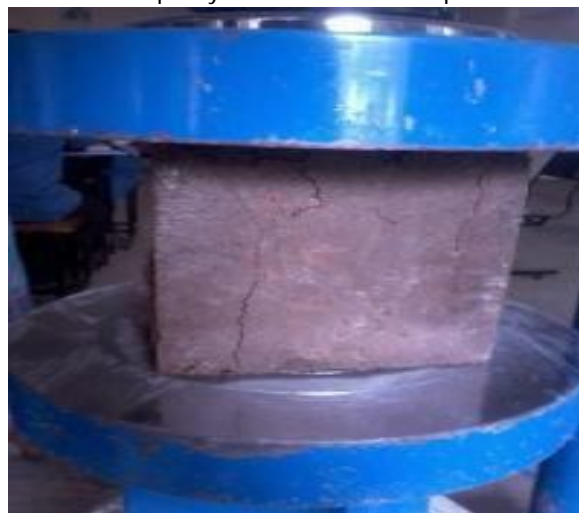
Fig: Testing of cube specimen for compressive
