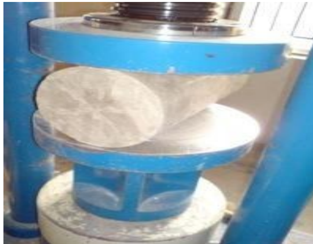
Fig: Testing of Cylindrical Specimen for Split Tensile Strength
