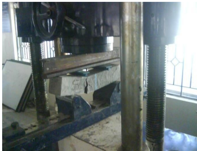
Fig: Failure Pattern of Beam in Flexural Strength Test
