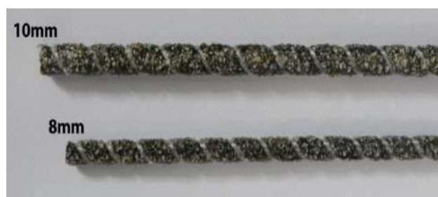
Figure-1. BFRP bars of different diameters
