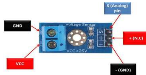
Fig 6. Voltage Sensor Pin Configuration
