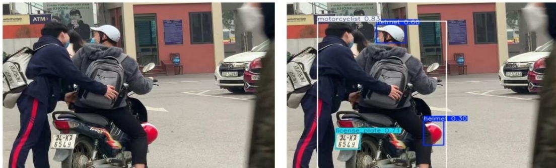
Fig 6: License Plate and Helmet Detection with bounding boxes
