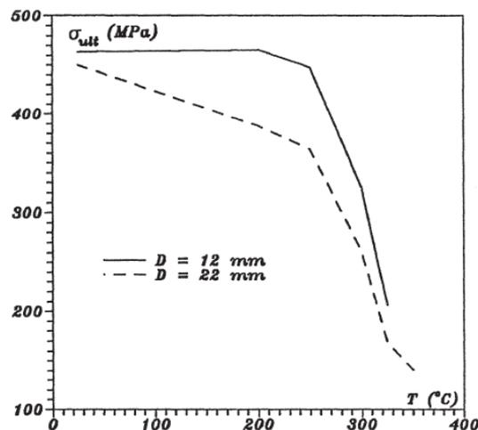
Figure 7: Variation of Ultimate Strength v/s Temperature
