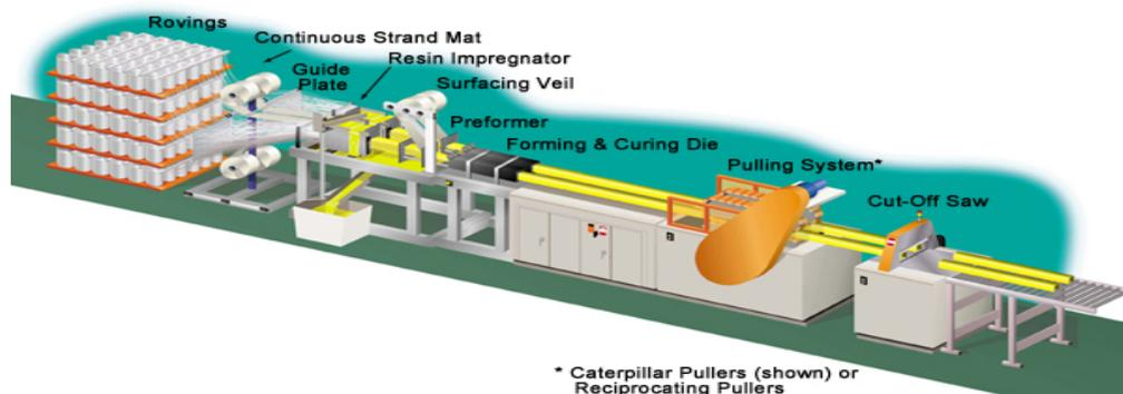
Figure 1: pultrusion process
