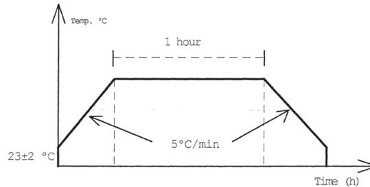
Figure 3: Variation of Temperature during the Exposure
