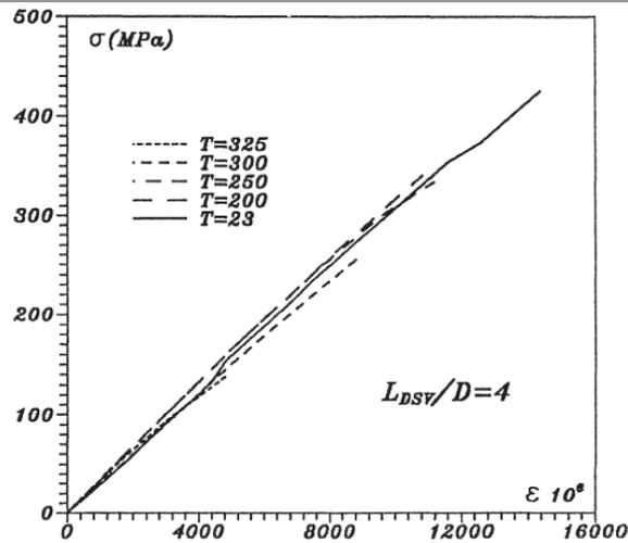
Figure 4: Stress- Strain curve for 12mm diameter
