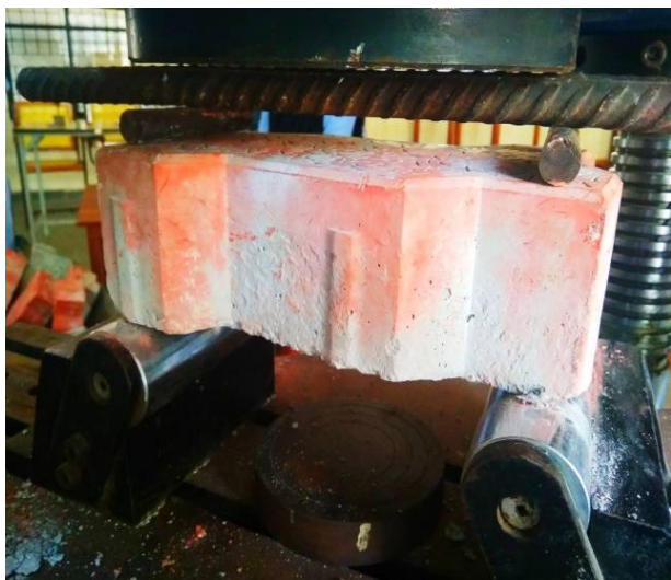
Fig. 4 Paver interlock loaded on UTM
