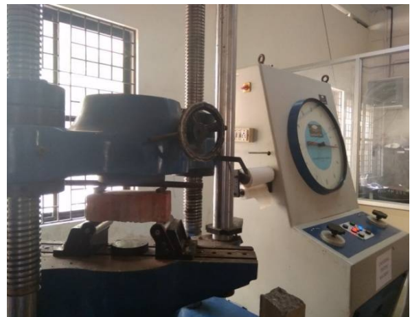
Fig. 3 Flexural strength test on paver interlock
