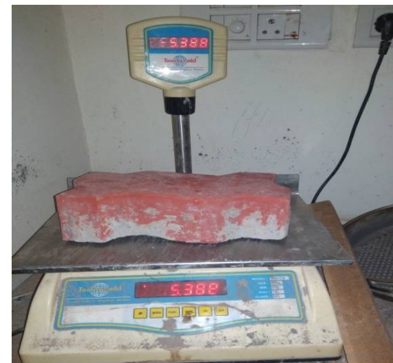
Fig. 5 Water absorption test on paver interlock
