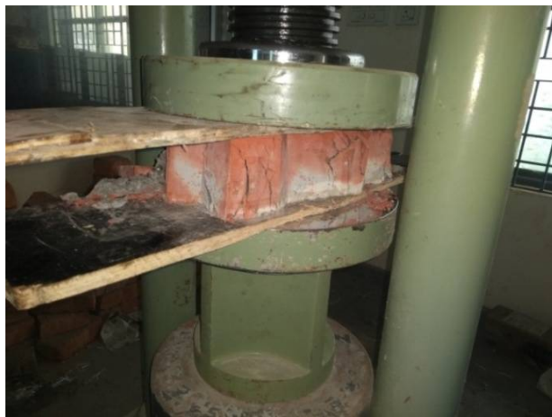
Fig. 2 Compressive strength test on paver interlock
