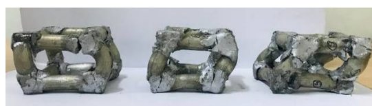
Figure-5: Aluminium solid rod lattice structures after test.
