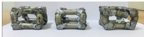
Figure-9: Aluminium solid rod lattice structures after dynamic test
