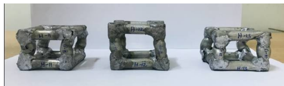
Figure-10: Aluminium tube lattice structures after dynamic test
