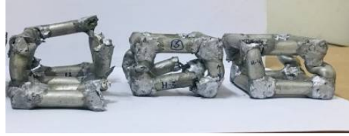
Figure-6: Aluminium tube lattice structures after test.
