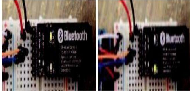
(a) Disconnected (b) Connected Figure 10: The Bluetooth connection status
