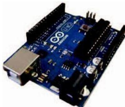
Figure 3: Arduino controller
