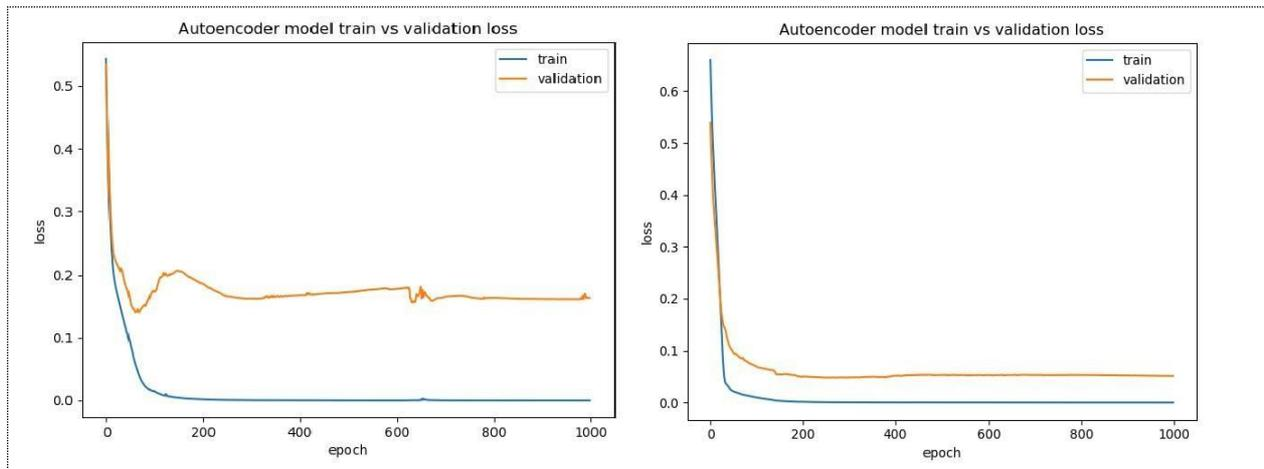
FIGURE 8. Loss graph for Autoencoder model (a) Simple AE model (b) Wavelet AE model
