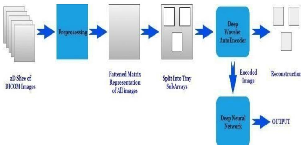
FIGURE 1. Proposed architecture of a DICOM image classifier for brain disease detection based on DWA-DNN model
