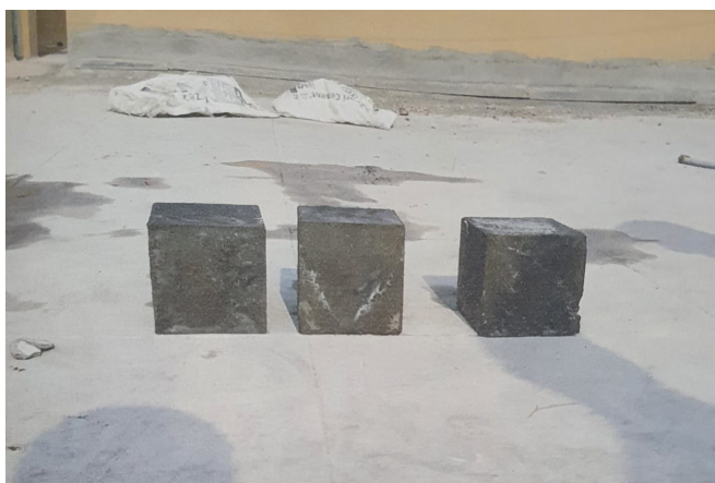
Fig. Cubes after 7 days of curing
