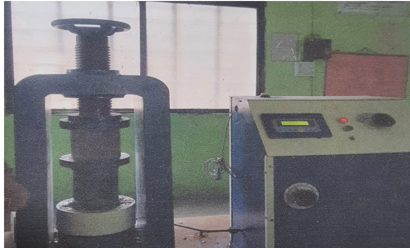
Fig. 6 Compression testing on cubes
