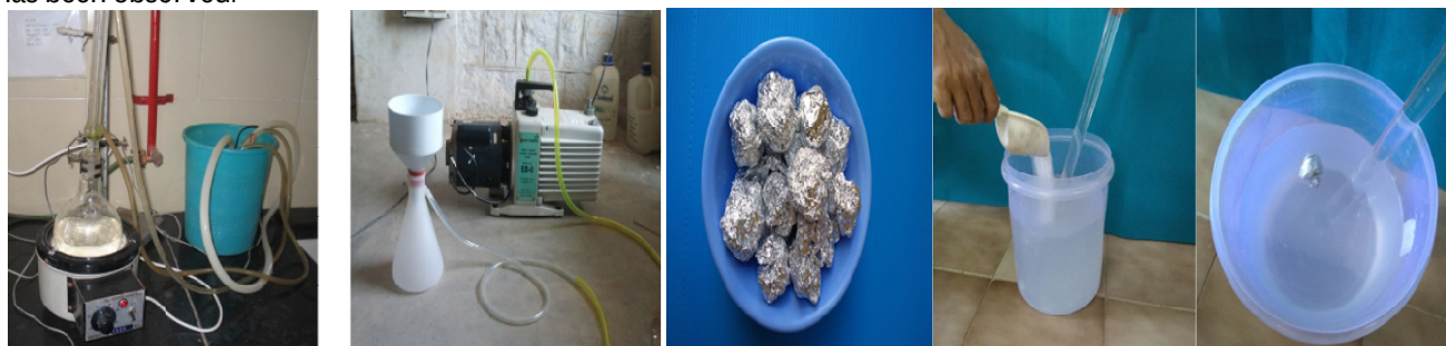
Figure: (a) Refluxing Setup & (b) Vacuum filtration setup (c) Aluminum balls (60g), (d) Sodium hydroxide solution, and (e) Dissolution of Aluminum foil in NaOH.
