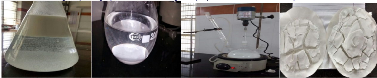
Figure 6.5: Photographs of (a) White-colored residue of [NaOH + ZnOAc], (b) Clear solution of NaOH with ZnOH precipitate at the bottom, (c) Refluxing set up, and (d) Dried Nano ZnO.
