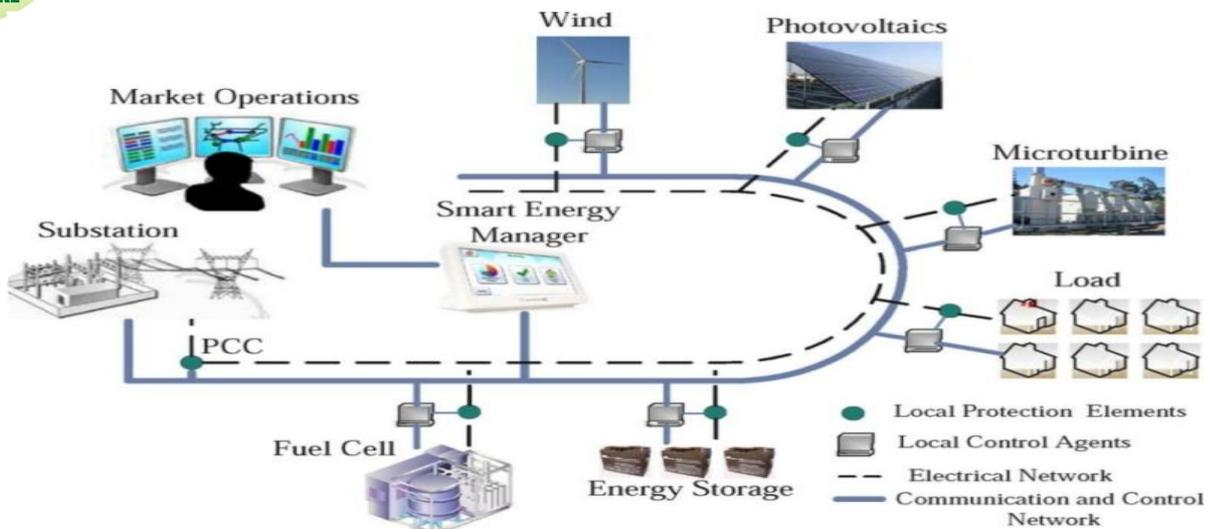
Fig-2 Microgrid Network Topology (Source: Google)
