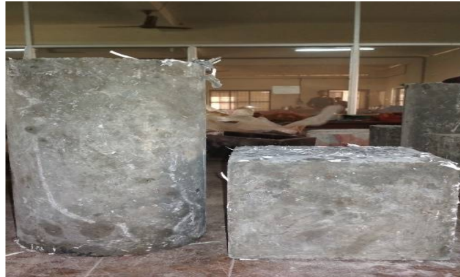
FIG.6 Plastic reinforced concrete
