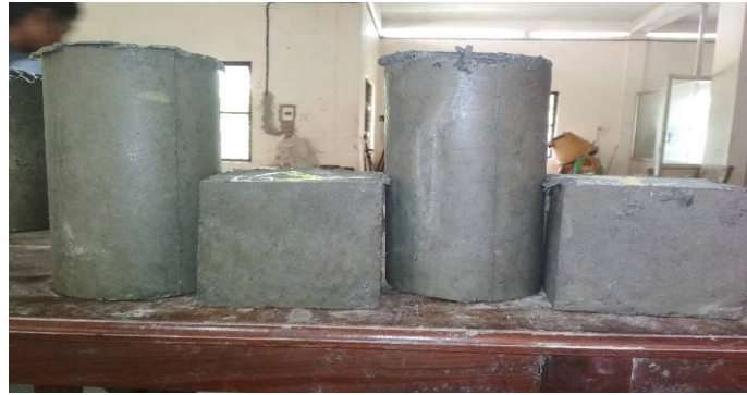
FIG. 2 Nylon reinforced specimen
