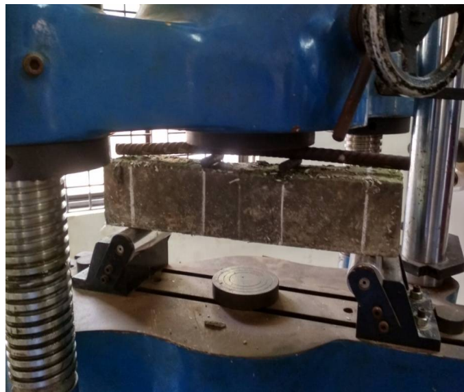
Fig.10 Flexural strength test on beams
