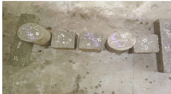
FIG. 4 Coir reinforced specimen
