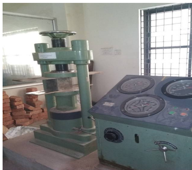
Fig. 8 Compressive strength test on cubes
