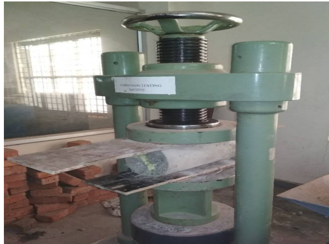
Fig. 9 Split tensile strength test on cylinders
