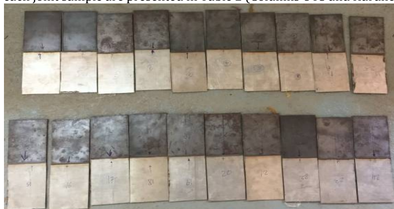
Figure 1. Weld joints of the dissimilar metals
